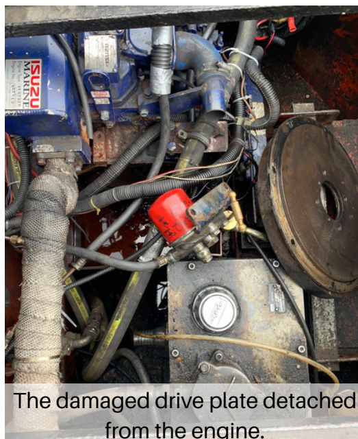
The end of the engine with the drive plate removed.
